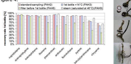
**Figure 4:** Transmittance of a heated filter (particulate filter @ 180°C, 200l/h gas flow, without carbonous dust or other)
