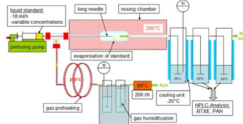
**Figure 3:** Test gas generator concept used, right test object
