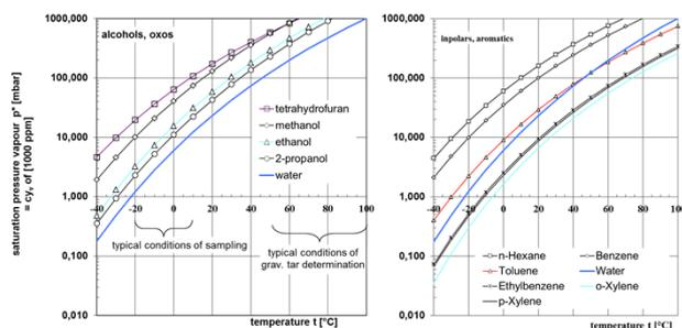
**Figure 1:** Saturation pressure of typical solvents for liquid sampling
