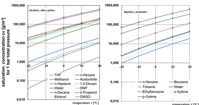
**Figure 2:** Calculated solvent losses for saturation, total pressure 1 bar.
