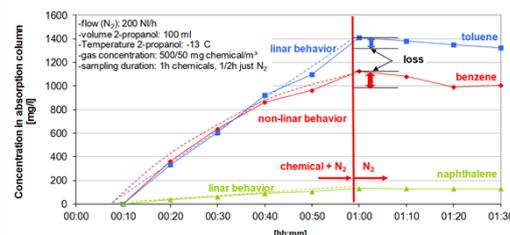
**Figure 5:** Dynamic test in a 1-stage impinger setting
