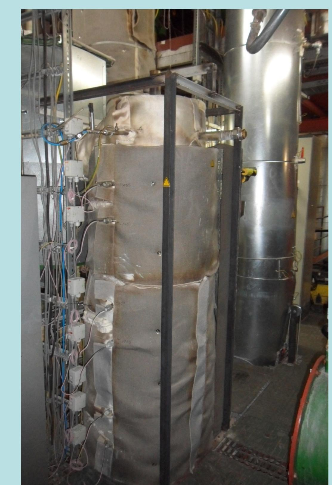
5 kW<sub>th</sub> lab-scale gasifier
