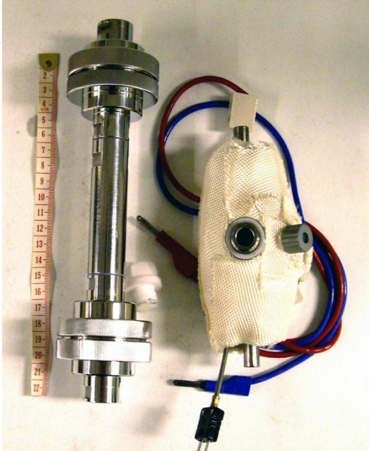
The T-joint allows simultaneous light tar analysis via septum (SPA) and connection to sampler for heavy tar analysis (by weight).
