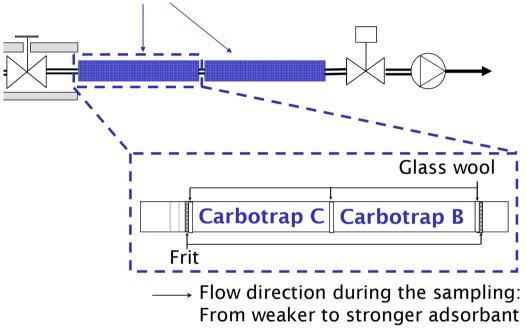
$\longleftarrow$  Flow direction during desorption
