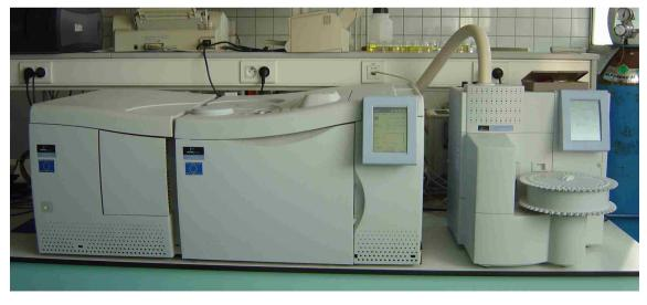
ATD coupled to Perkin Elmer GC/MS-FID
