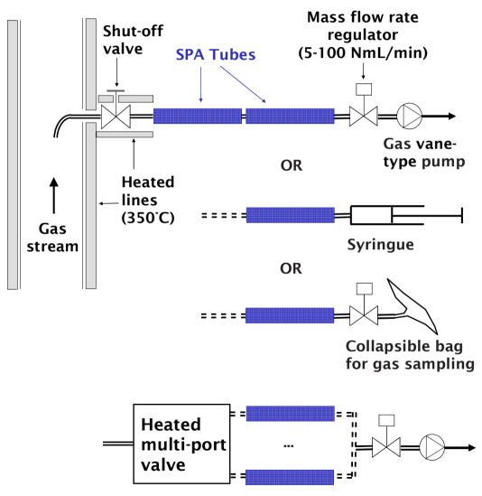
Sampling time (seconds to minutes): depending on expected concentration and adsorption breakthrough volume of adsorbent for each tar
