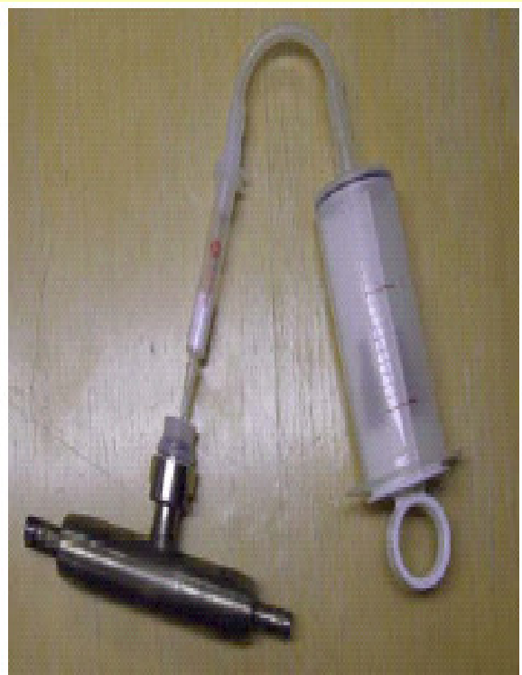
“T”, needle, SPE-NH2 tube and syringe 100ml.
