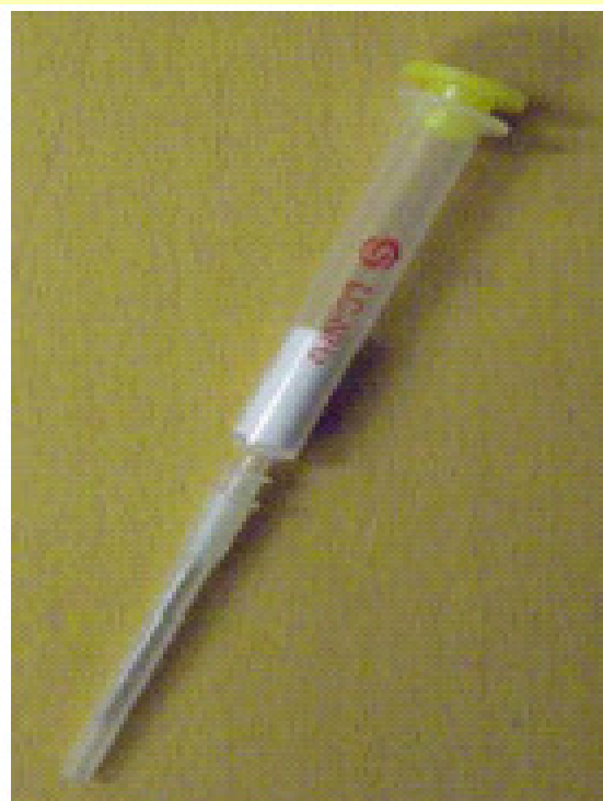
The SPE tube is capped in both ends after sampling.
