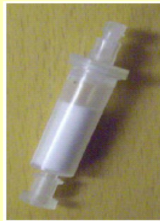
Custom made reversible SPE tube, it consists of a female Luer inlet and a Luer male outlet.
